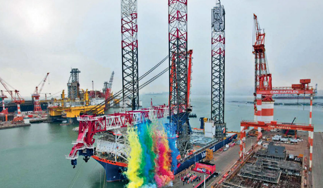
The offshore installation vessel measures 175m in length and has a 155-m high boom, which can lift more than 3,000 tonnes
