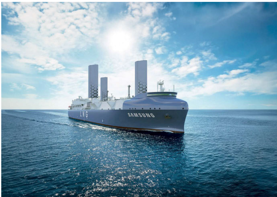
Illustration of the wing sail-equipped LNG carrier design
