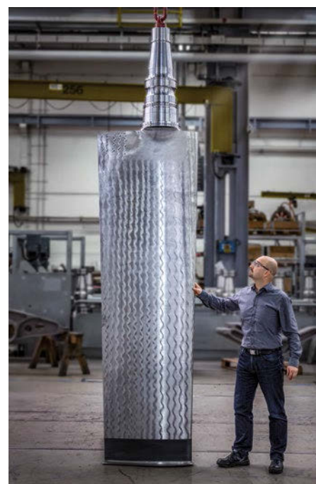
Figure 3: Blade size of a modern VSP (4-MW VSP unit)
