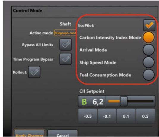
The system is optimised to ensure the best combination for engine RPM and propeller pitch resulting in minimised fuel consumption Source for both images: Qtagg
