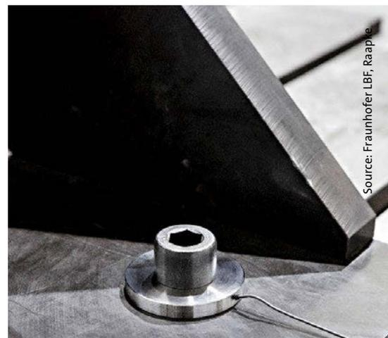
The force-measuring washer based on Delta-C® technology from Fraunhofer LBF can be used for monitoring wind turbines
