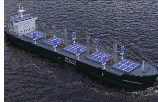
The Aquarius Eco Handymax II bulk carrier design is all electric and is equipped with fuel cells
