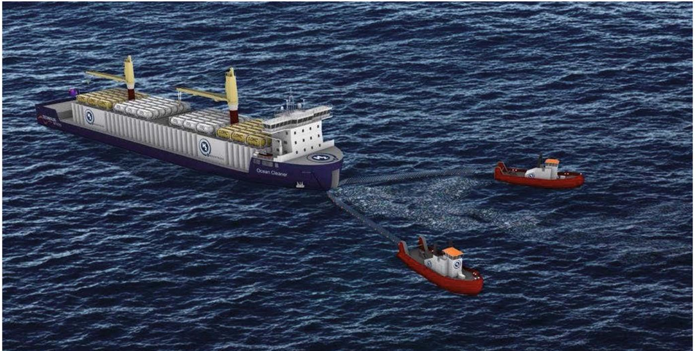
The ship will travel at four knots with the waste plastic collected by two smaller vessels towing a two-mile net that funnels the waste from the surface to a depth of 10m
