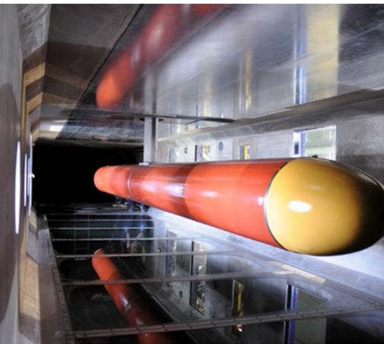
Figure 3: Torpedo-shaped test setup for friction measurements. Picture taken during friction measurements for the AIRCOAT project.
