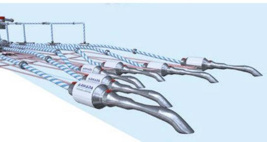
Rendering of the Armada Technologies air lubrication system
