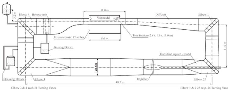
Figure 1: Schematic depiction of the Hydrodynamics and Cavitation Tunnel (HYKAT)
