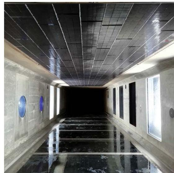
Figure 2: Flat plate setup for friction measurements. Here the surface is covered with AIRCOAT foil.
