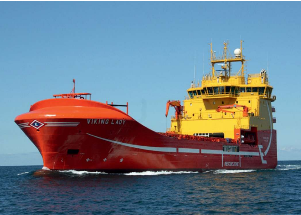
Eidesvik Offshore's Viking Lady became the first ship to be fitted with a 330kW fuel cell as early as 2009
