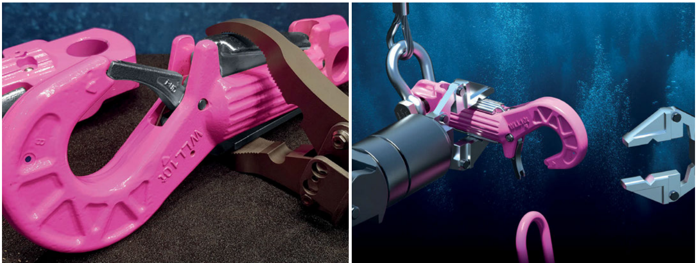
The lever mechanism of the ROV-Hook (left) is designed in such a way that its locking mechanism cannot be opened by one-sided impacts or blows. Instead, the hook can only be released by operating two levers in parallel, either by hand or, below water, by the ROV manipulator (right). Source for both images: RUD
