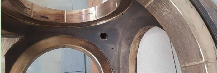
The use of biodegradable oil in CPP can attack metals. Piening has carried out many such overhauls for different brands
