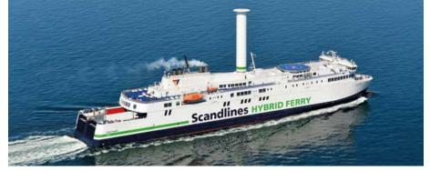
Norsepower Rotor Sails installed on Scandlines' vessel Copenhagen Source: Norsepower Oy Ltd
