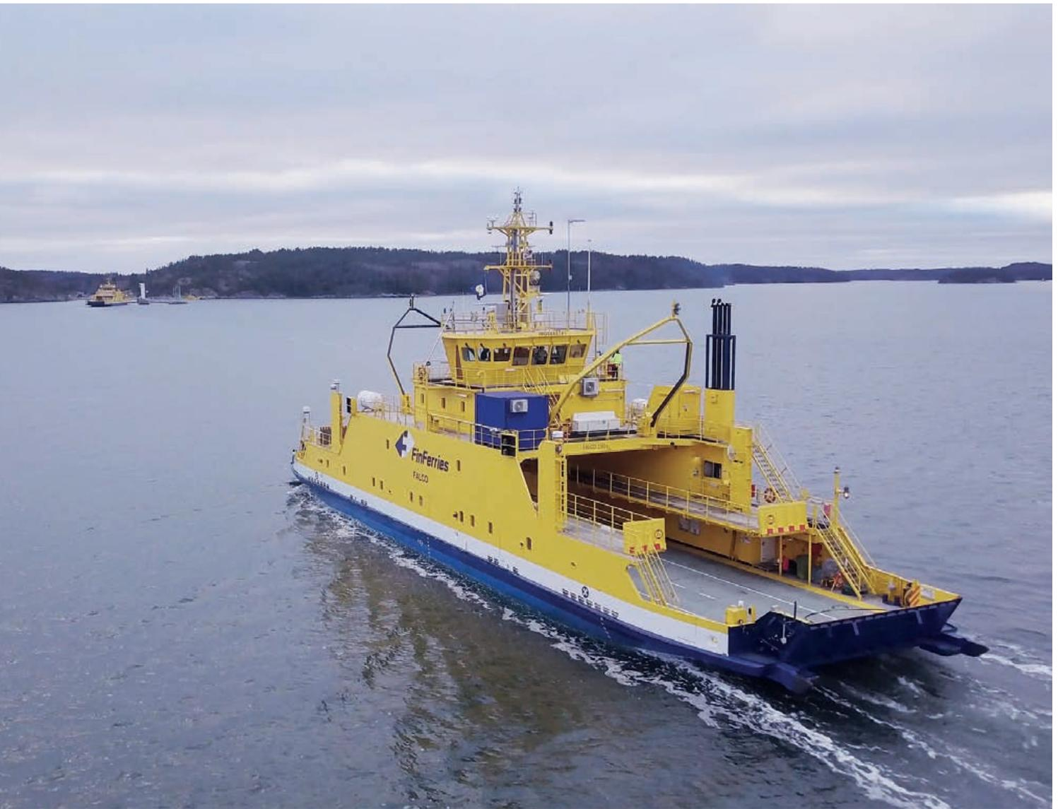
The *Falco* is a 53.8m-long double-ended car ferry, which entered service in 1993. It is equipped with twin azimuth thrusters from Rolls-Royce.
