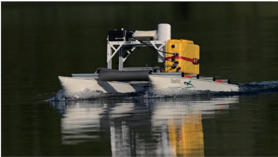
The SeaML is a development by Fraunhofer to test and verify promising technologies for maritime services. Within RAPID, the current setup will be modified and equipped with a landing platform and a battery hot swap system for UAVs.
