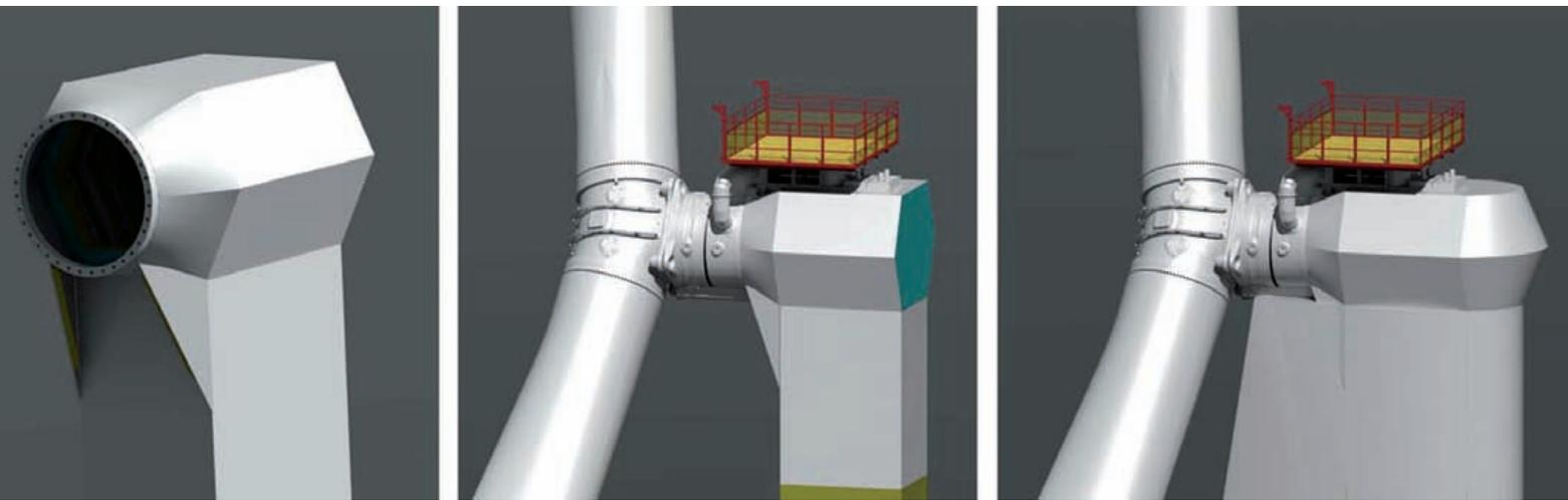
Figure 3: Tower head design, with and without aerodynamic cladding made of fibreglass
