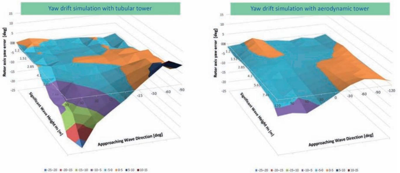
Figure 6: Yaw drift dependent on wind-wave offset with round (left) and profiled tower (right)
