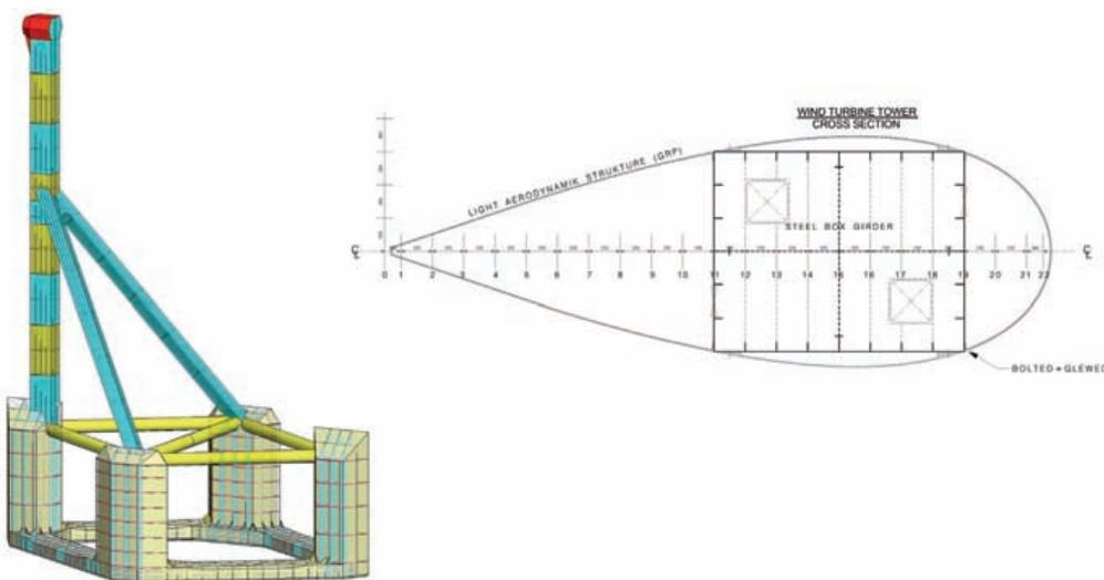
Figure 7: Optimised design: structure (left), the cross-section of the tower (right)
