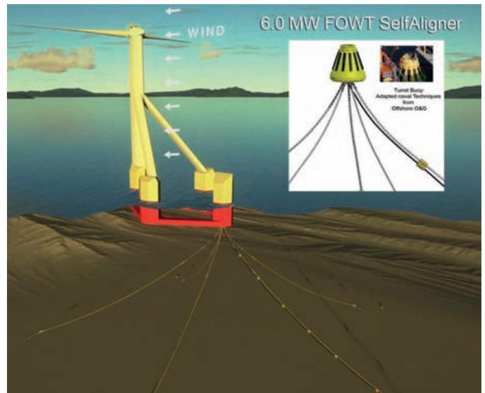
Figure 2: Design of the SelfAligner FOWT
