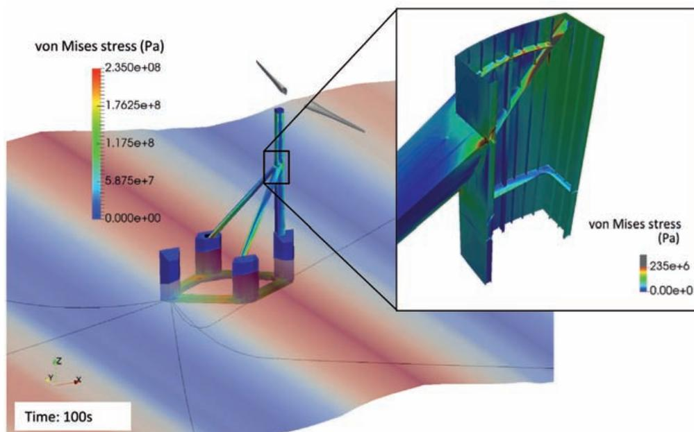
Figure 5: Simulation of FSI and stress analysis with detailed FE model
